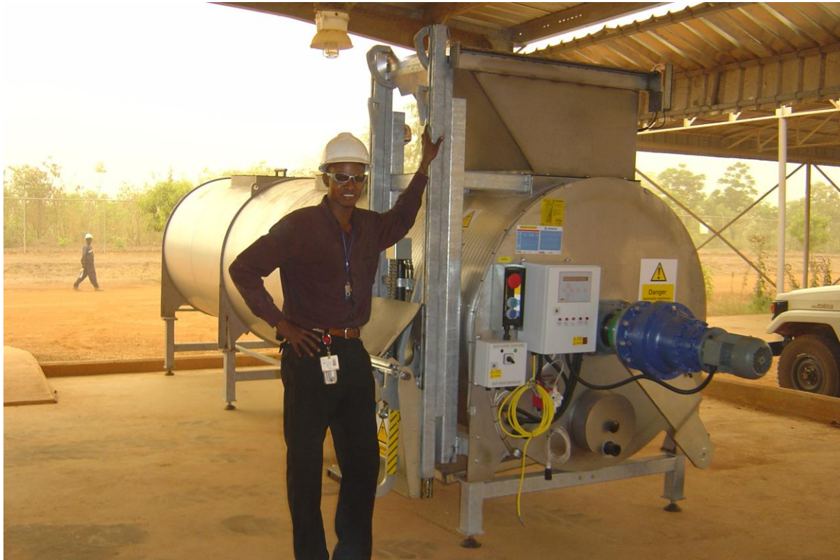
The A1200 Rocket Pictured with optional bin loading system, located at an Exxon oil exploration site in Africa, processes the food wastes generated from staff catering at the camp. The compost to be used in enriching the soils around the site.
